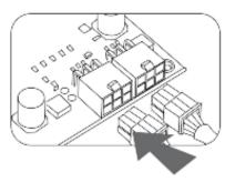
11 Connect your case fans to the regular 4-pin peripheral connectors if you are using these fans.
